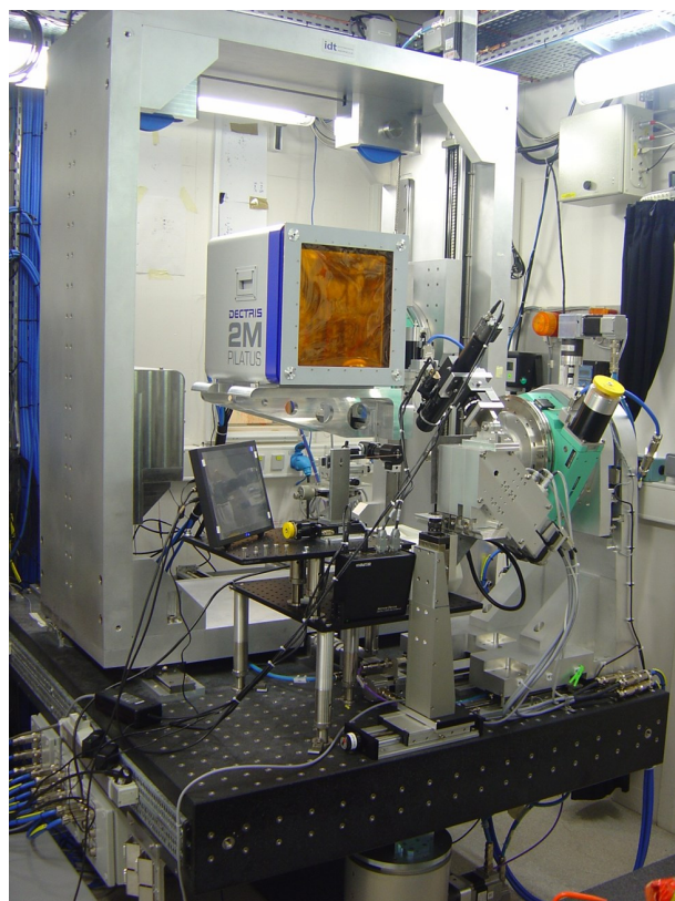
Above: Diffractometer detector mount installed on Swiss-Norwegian beamline at the ESRF.
