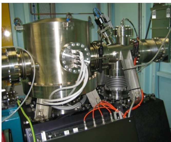
Above: Quad diode & secondary source aperture assembly installed on XFM beamline at the Australian Synchrotron.
